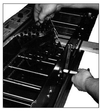
Figure 3-3. Removing the Turner Assembly.
