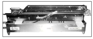
Figure 3-1. Draining the Shortening off of the Conveyor.
