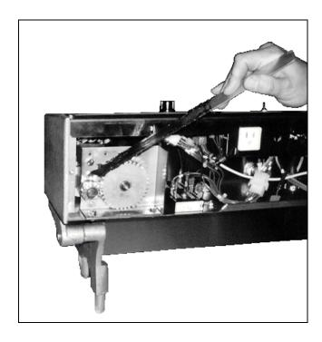
Figure 2-3. Lubricating the Drive Gears.
