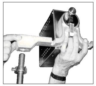
Figure 1-5. Mounting the Cutter Head Assembly.
