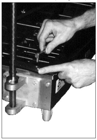
Figure 1-4. Connecting the Swing Connecting Rod.
