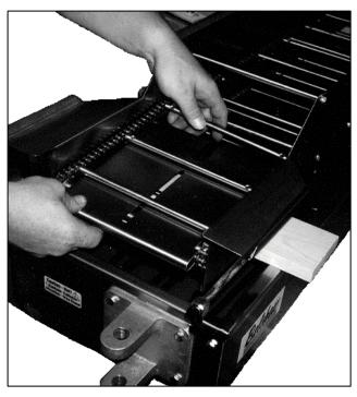
Figure 3-4. Removing the Drop Plate.
