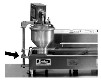
Figure 2-2. Lubricating the swing column.
