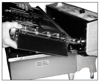
Figure 1-2. Joining the Couplings.
