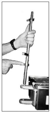
Figure 1-3. Inserting the Swing Column.
