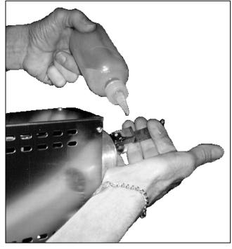
Figure 4-1. Lubricating the Connecting Rod.
