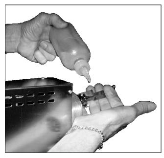
Figure 2-1. Lubricating the Connecting Rod.
