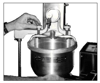
Figure 1-6. Mounting the Hopper.
