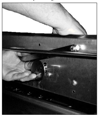
Figure 3-2. Removing the Turner Cam Assembly.
