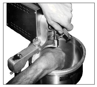
Figure 1-7. Installing the Plunger.
